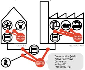
Data measured by Energomaster is sent via a communication interface (optional LTE, WiFi, LoRaWAN, etc.) to monitoring and management systems at adjustable intervals (5 seconds – 60 minutes). The MQTT and CoAP standards are used for data transmission.
